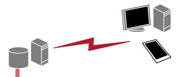
Access the Server PC (web server) using any PC or tablet with a web browser, and check equipment\*\* status and performance
